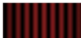
Interference from two narrow slits
