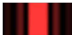
Diffraction from one (wider) slit
